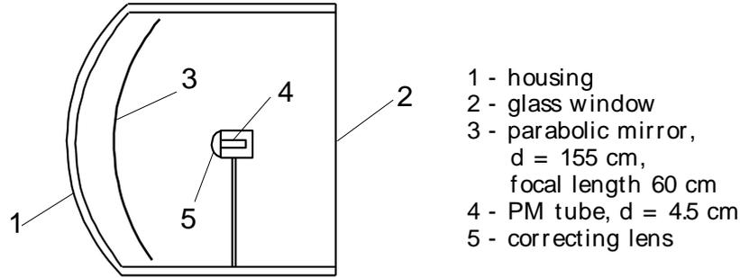
Fig. 1. The light receiver for Katsiveli experiment.
